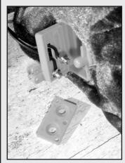
Figure 4. The external wire soldered to the battery contacts.
